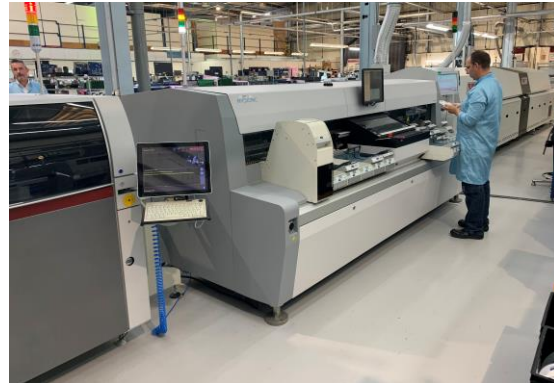
In line 10 zone Air/N2 Vacuum Reflow system
