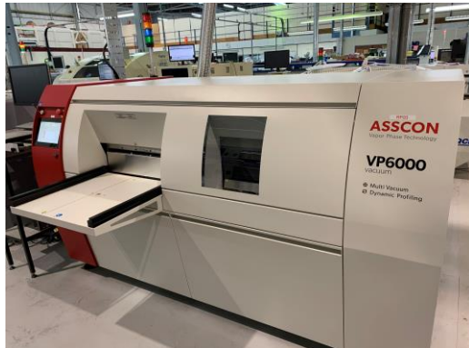
Vacuum Assisted Vapour Phase soldering
